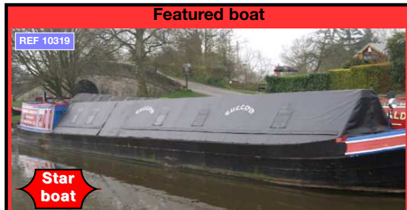
Featured boat REF: 10319 Rigal was built by the famous ship builders; who also built the Titanic, Harland and Wolff in 1935 for the Grand Union Canal Carrying Company. She was originally built as a composite (iron sides and wooden bottom) butty boat and was intended to be paired with Dorado. Her original butty stern was later removed and a conventional motor boat stern added and her wooden bottom replaced with a steel one. In 2005 she had a new back cabin, engine room and "under cloth" conversion constructed out of steel by Barry Hawkins at Atherstone. Rigal is presented in the Coronation livery of the Grand Union Canal Carrying Company of 1937. She is powered by a traditional Lister HA2 air-cooled marine diesel engine with Blackstone gear-box. Layout from the rear comprises of a traditionally decorated boatman's cabin and engine room. Her main cabin is then fitted out to a very high standard in solid Ash and comprises of a large open plan saloon with solid fuel stove, galley, bathroom and large double bedroom. The main cabin has portholes along its length, prisms in the top plank and three sets of side doors. She is heated by a solid fuel stove in the saloon. This boat benefits from a 5kVA onboard diesel generator, fridge, freezer, washing machine, inverter/charger making her an ideal liveaboard or luxury holiday boat. Rigal is licensed until February 2015.
